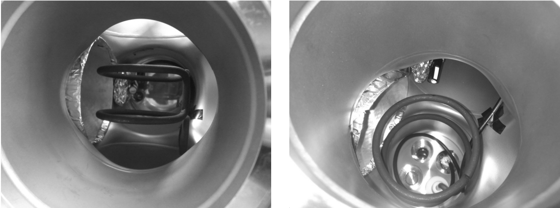
Fig. 11: Front and top view of the suppressor electrode as it was installed into the chamber
