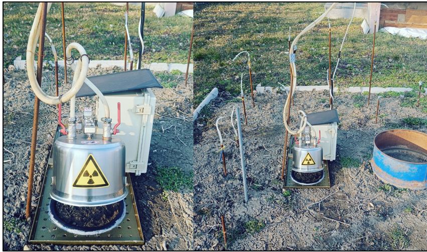
Fig. 1.3 Accumulation chamber setting for the measurement of radon and CO 2 fluxes at the campus of the Faculty of Mathematics, Physics, and Informatics, Comenius University (FMPI CU) in Bratislava, Slovakia.
