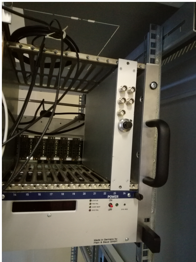
FIGURE 3.15: Photo of the custom signal converter as the NIM module in NIM crate.
