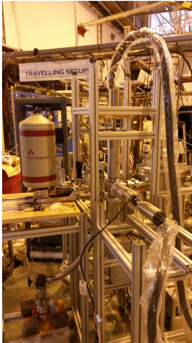
FIGURE 3.7: Photo of TATRA spectrometer at ISOLDE LA1 beamline with all detectors mounted.
