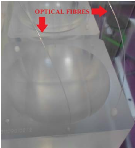
(a) Gluing of optical fibres.
