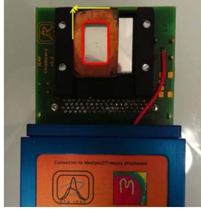
Figure 3.14: Alignment of the measured source on the detector. Sources in all the measurements were aligned with the top left corner of black plastic holder as depicted by yellow arrows. The relative position of the red Copper frame window and the top left point were known thanks to the previous measurements of the source dimensions listed in the Tables 3.1 and 3.2.
