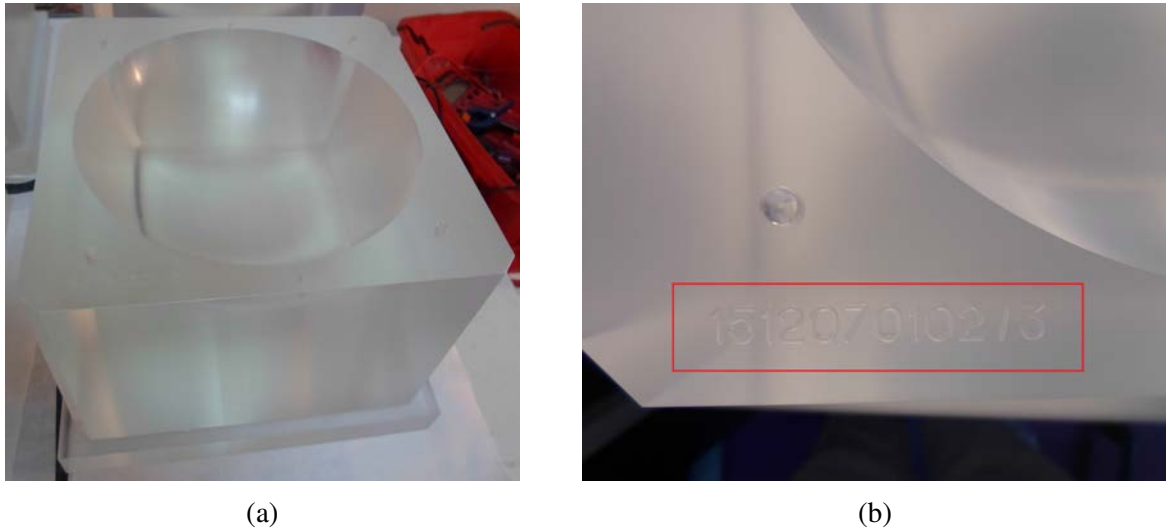
Figure 2.7: (a): Picture of real PS block produced by NUVIA. (b): Production number placed on top of each block.
