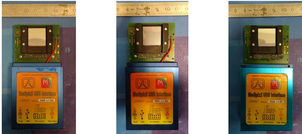
Figure 3.4: Photos of the Timpepix pixel detectors used in the study. From left: H04-W0163 (300 \mu\text{m} Silicon sensor), H11-W0163 (300 \mu\text{m} Silicon sensor) and L05-W0163 (1 mm Silicon sensor). The chip is located in the top part of the detector, lower, blue part is USB interface developed in IEAP CTU in Prague [78].
