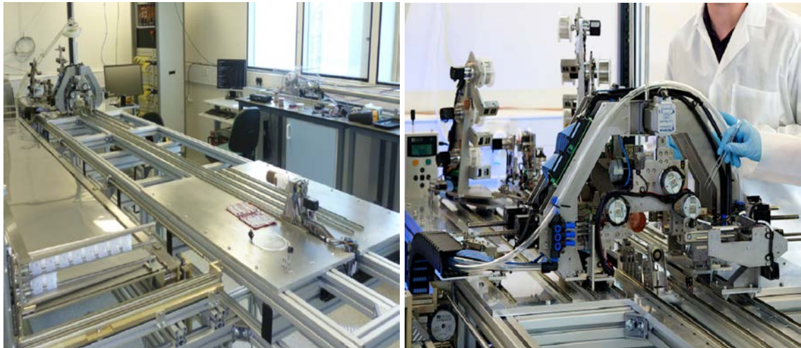
Figure 2.4: Photos of robot developed for the preparation of the tracker cells.
