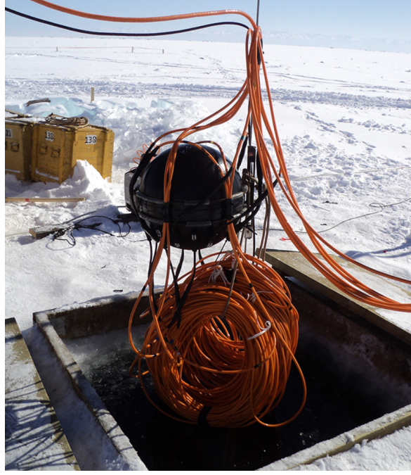
Figure 2.7: Central module attached to a string. There are 12 copper cables in orange coating that connects each OM with the CeM. Image credit: Baikal-GVD Collaboration.
