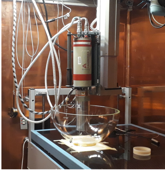
Figure 3.9: Experimental setup for measurements of the DOM glass radioactivity in National Radiation Protection Institute in Czech Republic. For estimation of the radioactive isotopes contribution HPGe detector was used.
