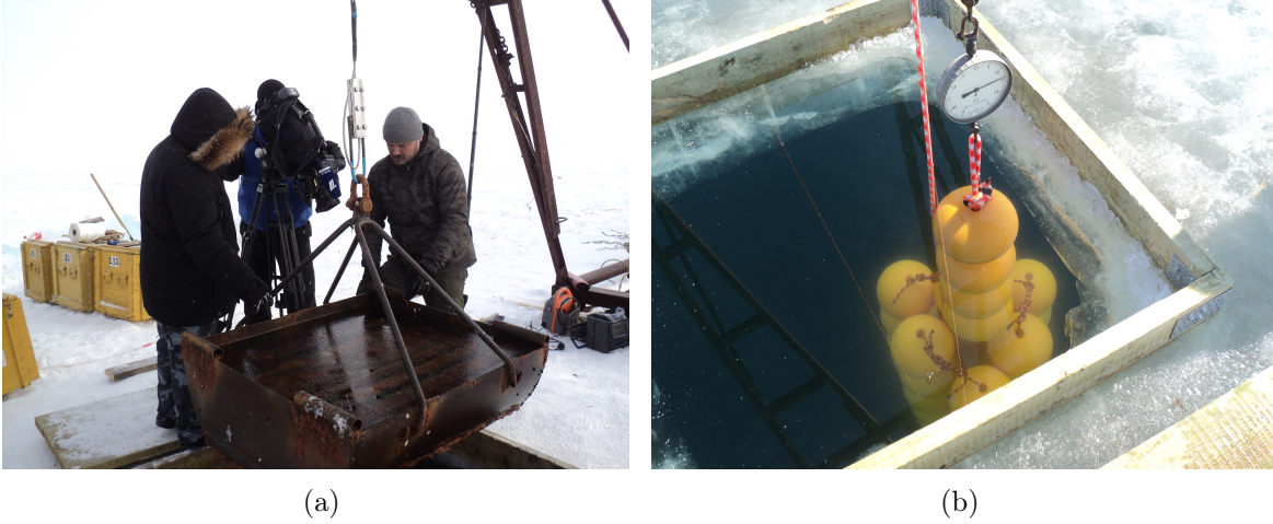
Figure 2.9: a) Photo of the anchor of the Baikal-GVD string. b) Photo of the buoys attached to the top of the Baikal-GVD string. Image credit: Baikal-GVD Collaboration.
