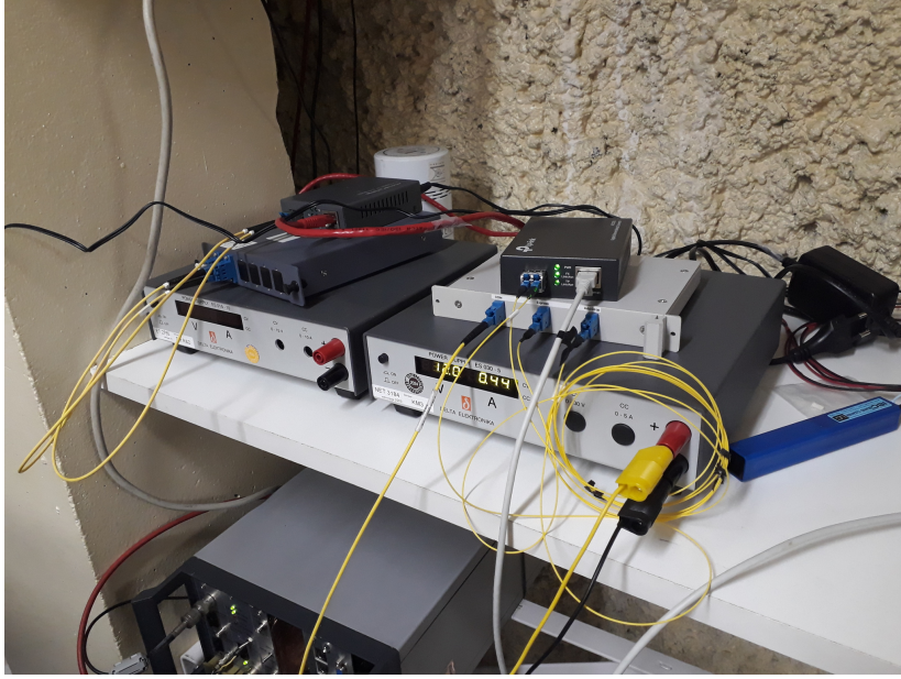
Figure 3.3: Photo of the electronics used for the single DOM measurements in the Modane underground laboratory.
