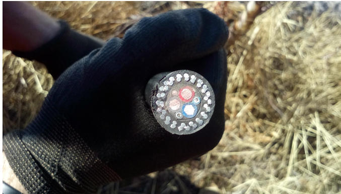
Figure 2.10: Photo of the electro-optical cable used in Baikal-GVD, that connects the DAQ cluster center with the shore station. Image credit: Baikal-GVD Collaboration.
