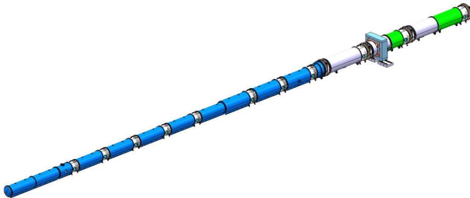
Figure 2.9: The NA62 vacuum vessel called the Blue Tube, [84]. The beam comes from the left. The white sections dividing the Blue Tube are individual LAV stations (subsection 2.2.5). The downstream spectrometer magnet can be seen as a light-blue square-shaped object downstream (subsection 2.2.3).
